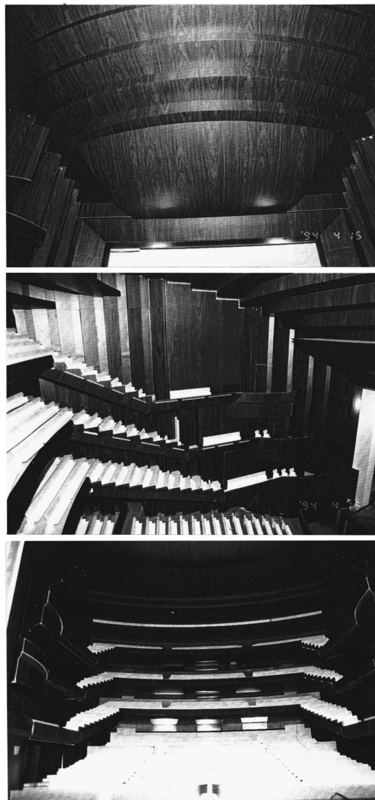
FIG. 2. Photographs of a late version of the 10:1 scale model of the NNT opera house.
