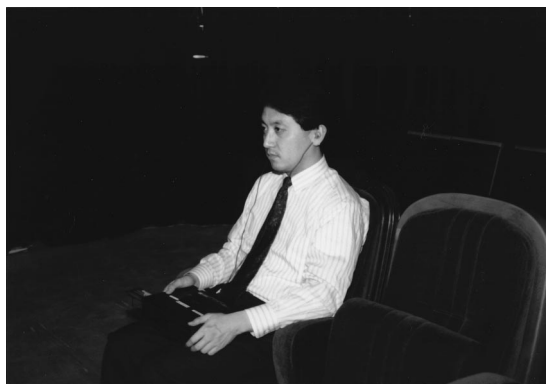
FIG. 2. Subject wearing miniature microphones at outer ear canals and DAT recorder in his lap for binaural measurements at audience positions.
