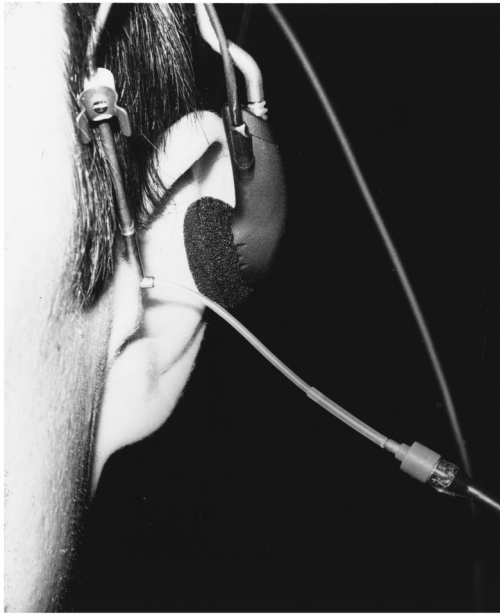
FIG. 1. Picture of a listener's ear with probe microphone and headphone.
